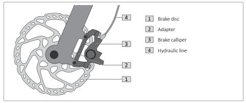
Fig. 5: Disc brake components
