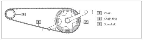
Fig. 2: Chain drive components
