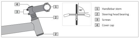
Fig. 13: Adjusting the handlebar stem (clamp with clamp screw)
