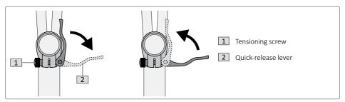
Fig. 17: Quick-release clamp
