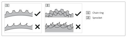
Fig. 3: Possible signs of wear on chain drive components
