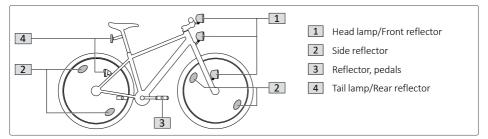
Fig. 16: Lighting components on the bike
