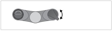
Fig. 15: Mechanical spring tension (left) and lock-out function (right) on the suspension fork
