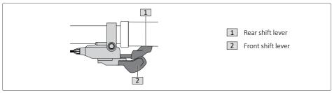
Fig. 6: Operating elements of the gear shift system
