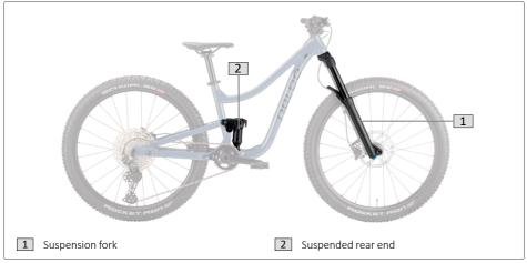
Fig. 14: Suspension components
